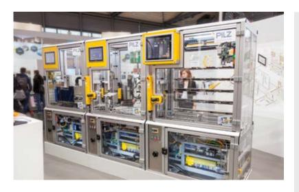
Automation of the future requires solutions that can distribute control intelligence and are still easy to use. The automation system PSS 4000 makes this possible. Multiple controllers with identical authorisation rights are connected simply via the real-time Ethernet SafetyNET p. SafetyNET p exchanges data and state information between the controllers and synchronises it.
