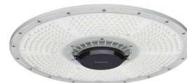
cloche LED 138W / 4000K / non dimmable / 90° / 20000lm / CRI 80 / gris PHI33568100
