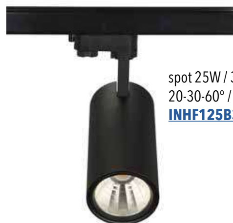
spot 25W / 3000K / non dimmable / 20-30-60° / 2375lm / CRI 90 / blanc INH125W3000
